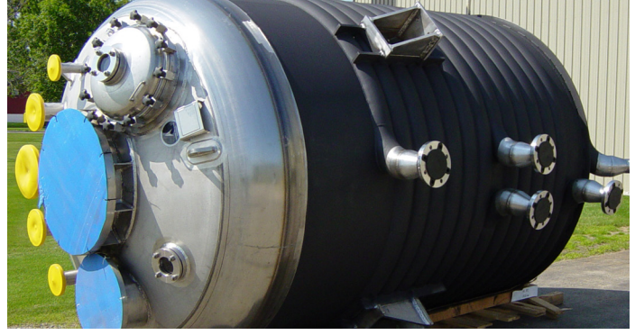
Heat reactor vessel showing ThurmaloX coating.
