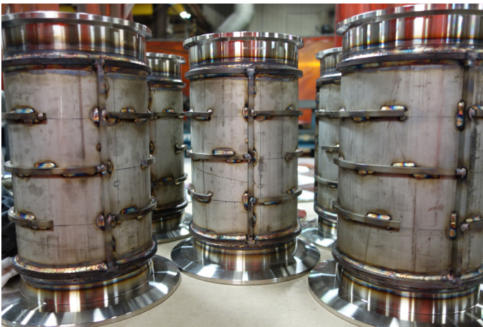
A row of small vessels showing channel weldments before the outer shell is added.
