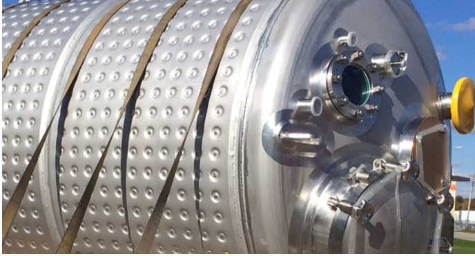
Pickle passivated dimple jacket prior to insulation.
