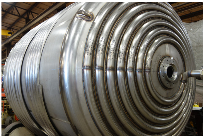
Tank showing half pipe construction.
