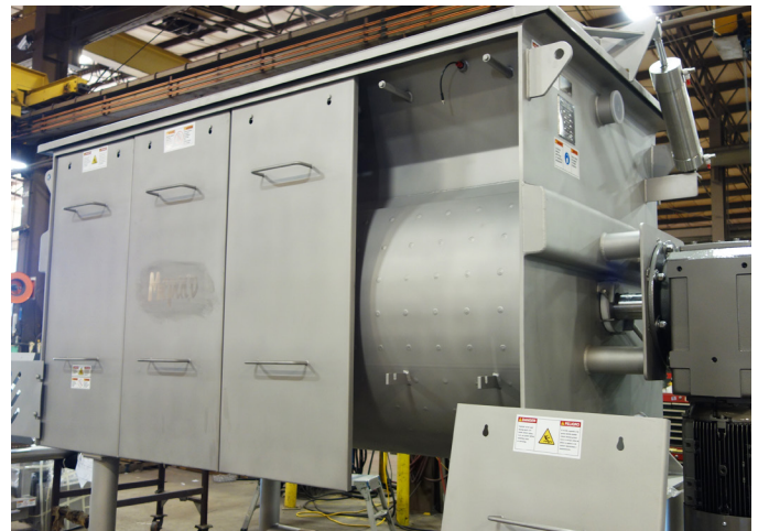
The heat shield removed on the ThermoBlend™ cooker exposing the stay bolt jacket.
