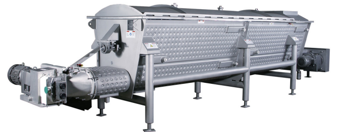
The auger cart is a pumping system that provides food product transfer between processes. The dimple jacket allows product to maintain required product temperatures during transfer.
